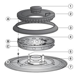
After cleaning the burner reassemble in the correct order:
